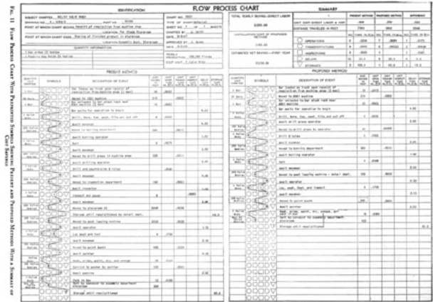
[Fig. 2] A variation of Flow Process Chart with pre-printed symbols. It shows the present and the proposed method, with a summary of cost savings. (Source: ASME 1947, 16. Public domain)
