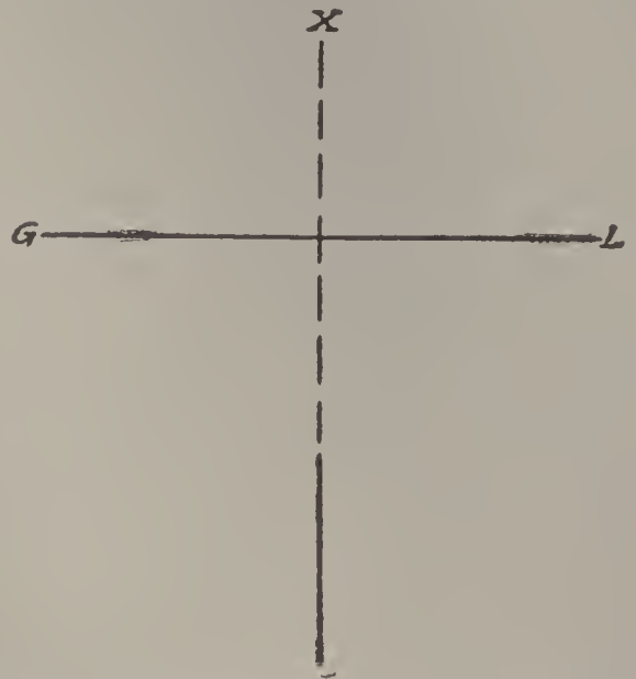
Fig. 116. Projections of a Line Perpendicular to Plane
