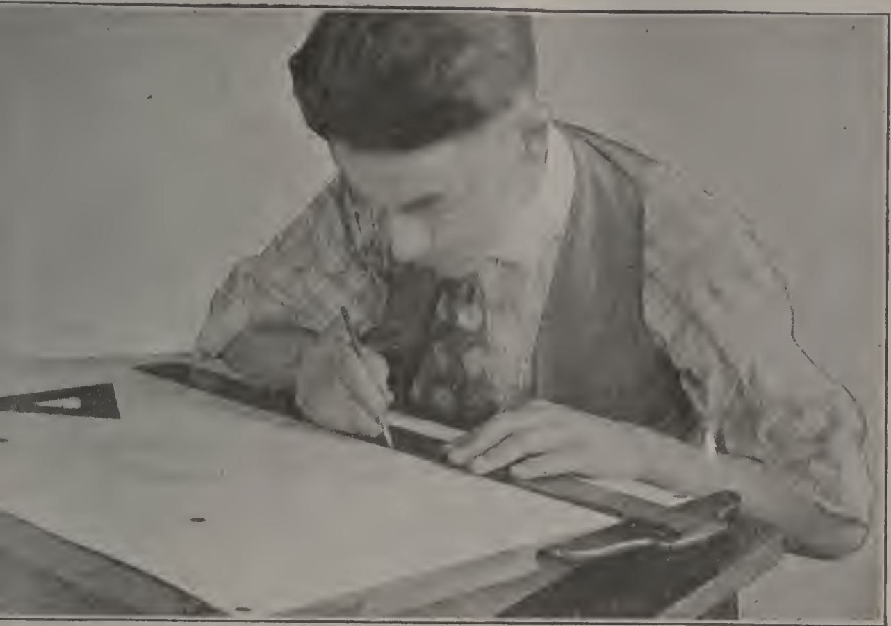
Position 3. Inking a Line with Pen and T-Square
