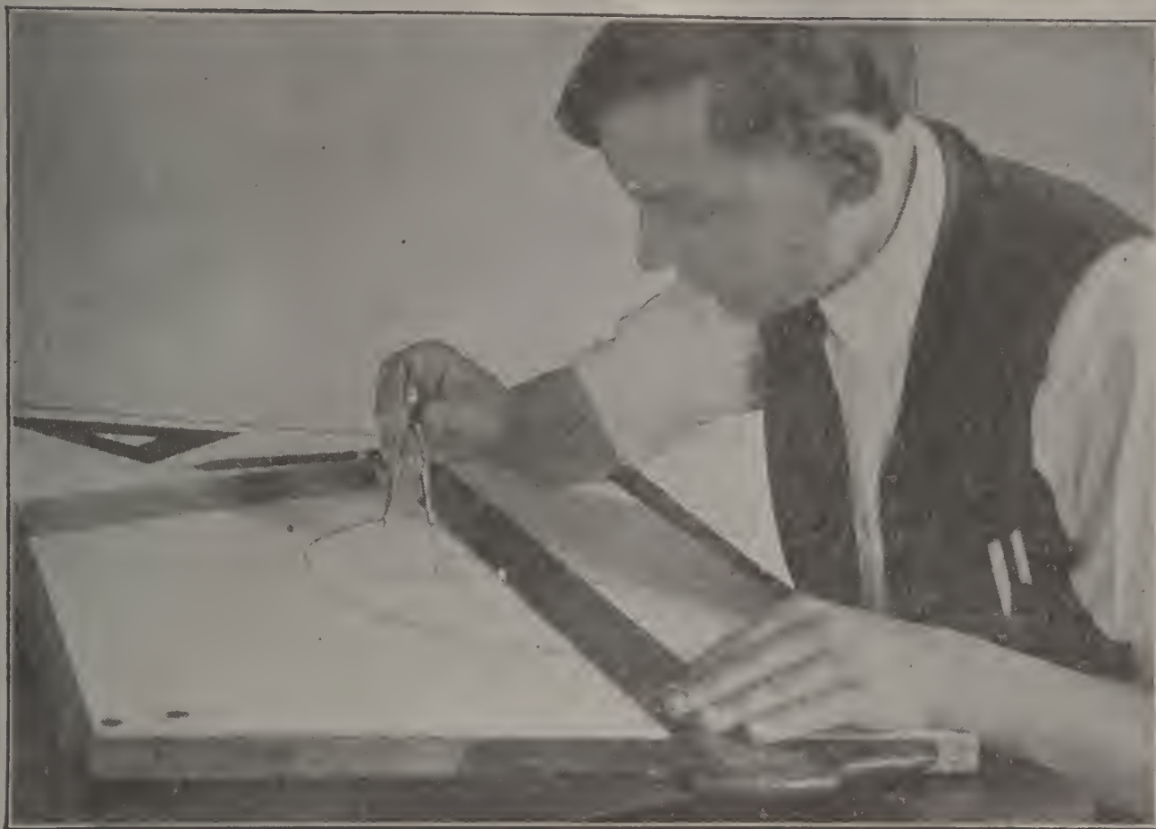
Position 7. Adjusting Dividers with One Hand. Note Second and Third Fingers between Legs
