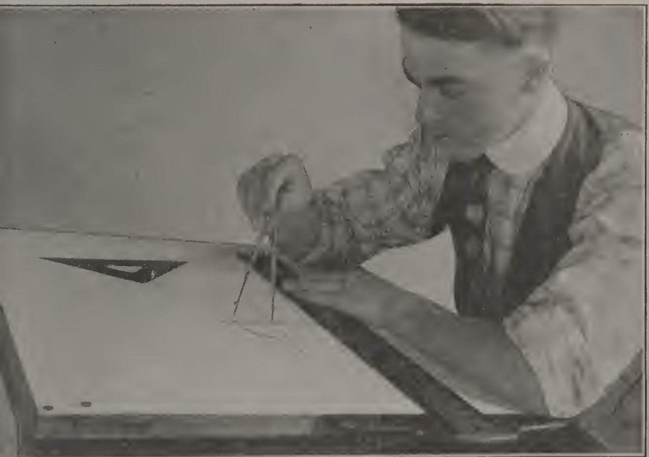
Position 4. Drawing Small Circle with the Compass
