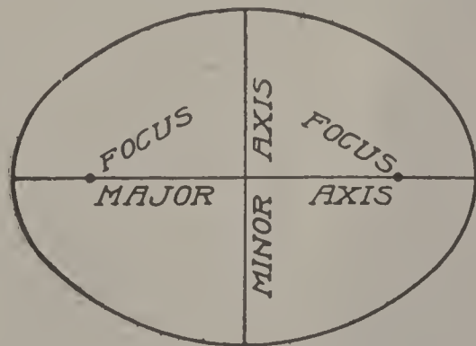
Fig. 86. Diagram Showing Constants of Ellipse
