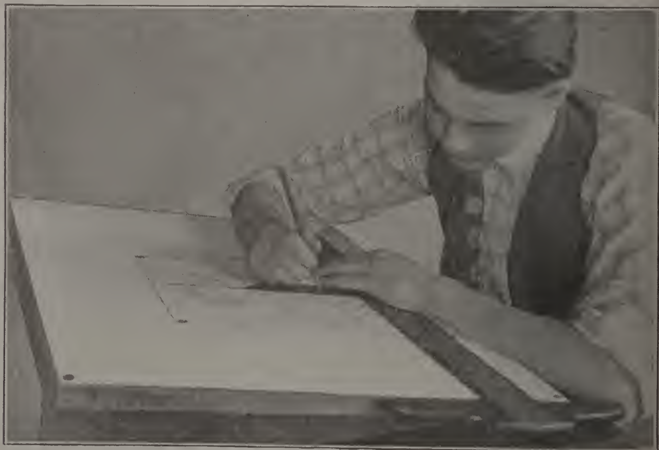
Position 2. Drawing Pencil Line with T-Square and Triangle
