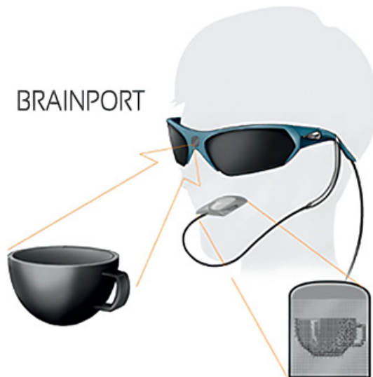
Figure 10 BrainPort. Device converting visual pictures into tactile sensations on the tongue, allowing users to “feel” the images.
